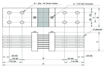
Thickness and gap of terminal blades are equal as 6.35mm.
