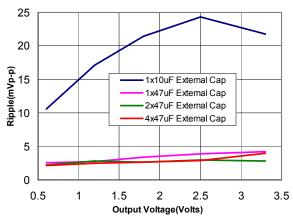
Figure A Output ripple voltage for various output voltage at Vin=5V, 6A load
