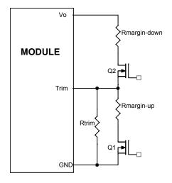
Circuit Configuration for margining Output voltage
