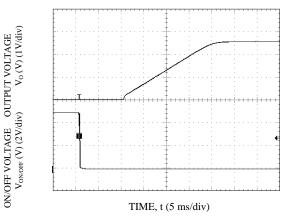
Start-up Using On/Off Voltage (Io = Io,max), Vo=2.5V
