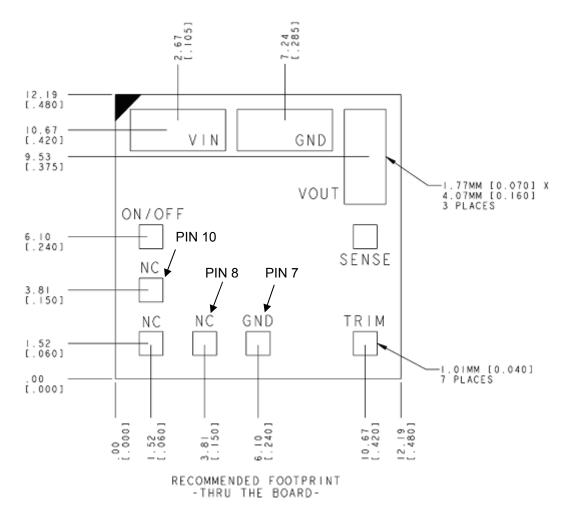
Dimensions are in millimeters and (inches). Tolerances: x.x mm  $\pm$  0.5 mm (x.xx in.  $\pm$  0.02 in.) [unless otherwise indicated] x.xx mm  $\pm$  0.25 mm (x.xxx in  $\pm$  0.010 in.)
