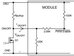
Circuit configuration for using negative On/Off logic
