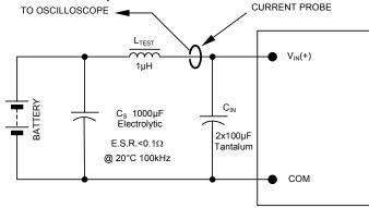
NOTE: Measure input reflected ripple current with a simulated source inductance ( $L_{TEST}$ ) of 1µH. Capacitor C<sub>S</sub> offsets possible battery impedance. Measure current as shown above.
