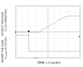
Start-up Using On/Off Voltage (Io = Io,max), Vo=1.2V
