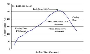
Recommended linear reflow profile using Sn/Ag/Cu solder.
