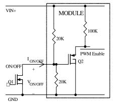
Circuit configuration for using positive On/Off logic
