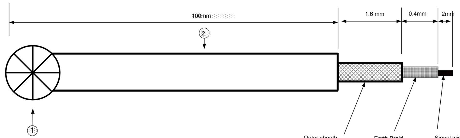
Outer sheath removed to expose the Earth Braid. Earth Braid is solder tinned
