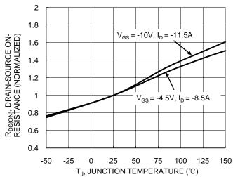
Figure 6. On-Resistance Variation with Temperature
