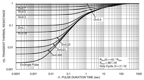
Figure 13. Transient Thermal Resistance
