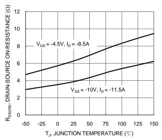
Figure 7. On-Resistance Variation with Temperature
