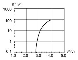
Fig. 3 Forward Current vs. Forward Voltage
