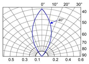
Fig. 2 Directivity Radiation Diagram
