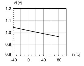
Fig. 5 Forward Voltage vs. Temperature
