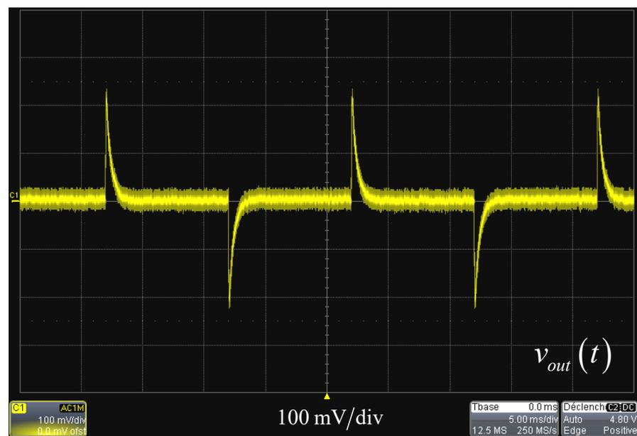
$$V_{in} = 48 \text{ V} - 5 \text{ to } 10 \text{ A} - 1 \text{ A}/\mu\text{s}$$
