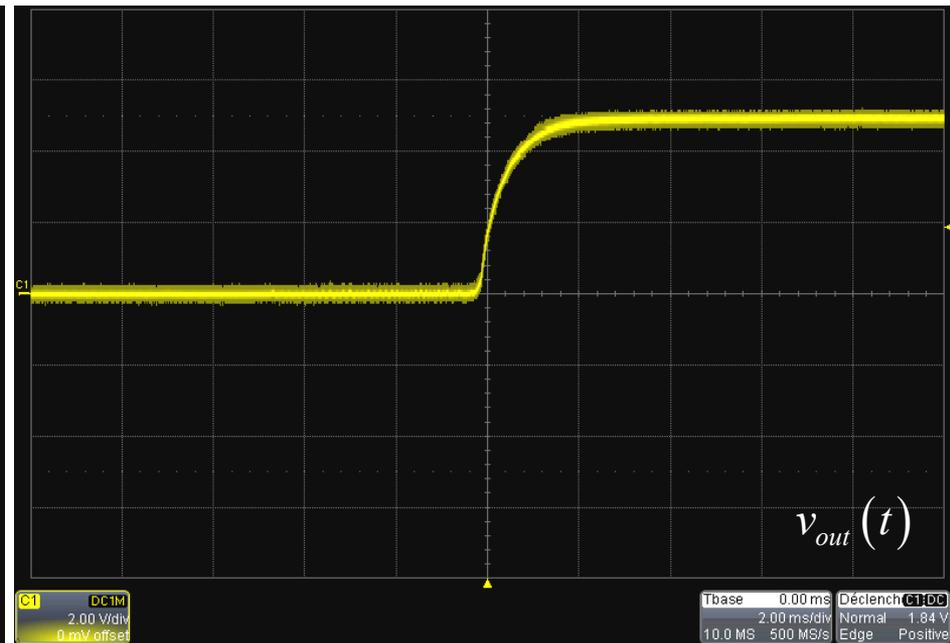
$$V_{in} = 0 \text{ to } 48 \text{ V} - I_{out} = 10 \text{ A}$$
