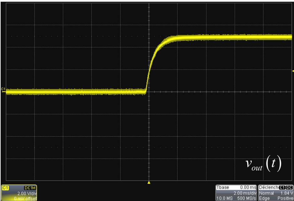
$$V_{in} = 0 \text{ to } 48 \text{ V} - I_{out} = 1 \text{ A}$$
