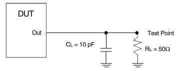
Load Circuit: Low-to-High Slew-Rate Adjustment
