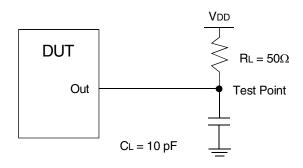
Load Circuit: High-to-Low Slew-Rate Adjustment
