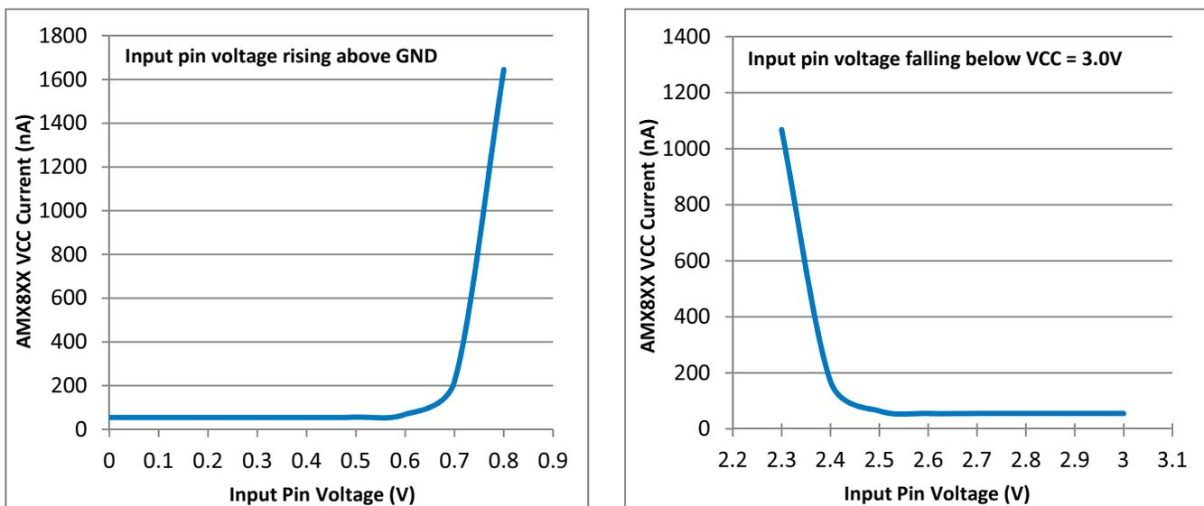
**Figure 5 – VCC Current and Input Pin Voltage**
