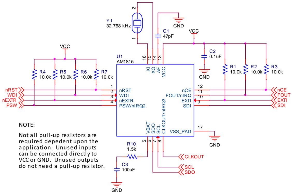
**Figure 9 – SPI Reference Schematic**
