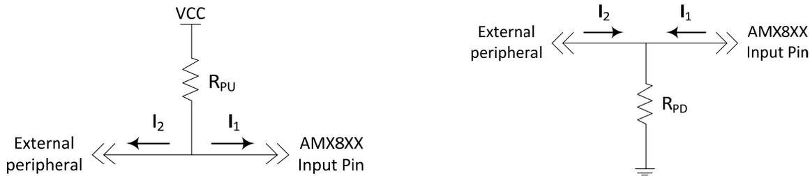
**Figure 4 – Pull-up and Pull-down Resistors**
