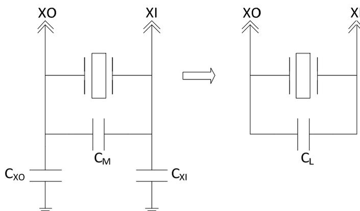
**Figure 1 – Crystal Circuit Schematic**
