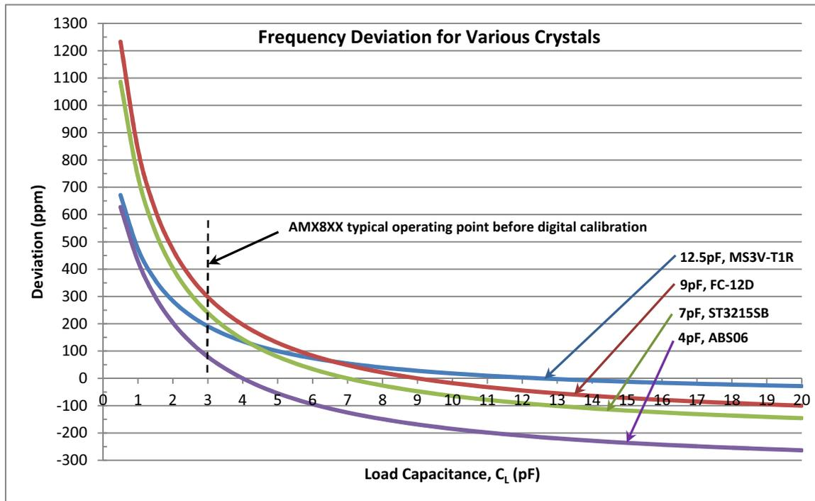
Even though the crystal oscillator circuit operates at a higher frequency due to the lower crystal load capacitance, the AMX8XX XT digital calibration feature allows the internal clocks to be calibrated to within +/- 2 ppm. The XT digital calibration feature has several benefits.
