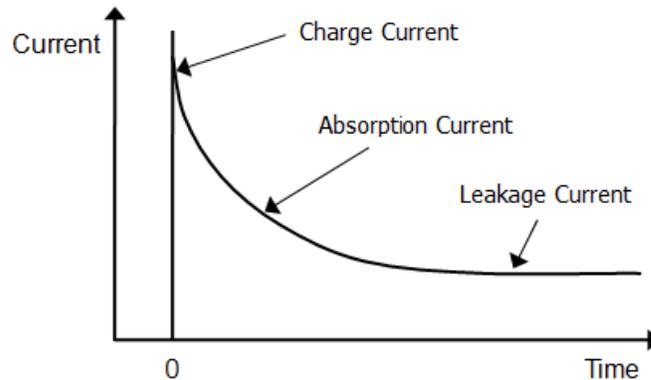
**Figure 7 – Ceramic Capacitor Current Profile**
