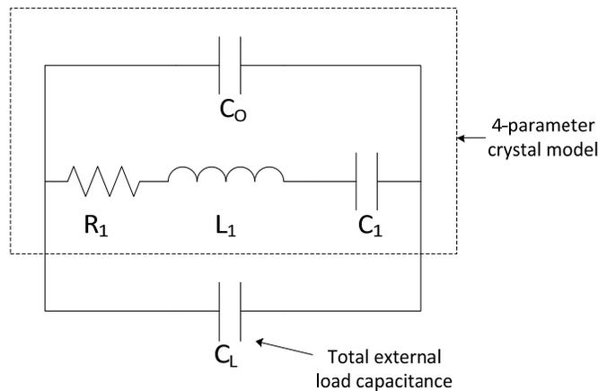
**Figure 2 – Crystal Circuit Schematic**
