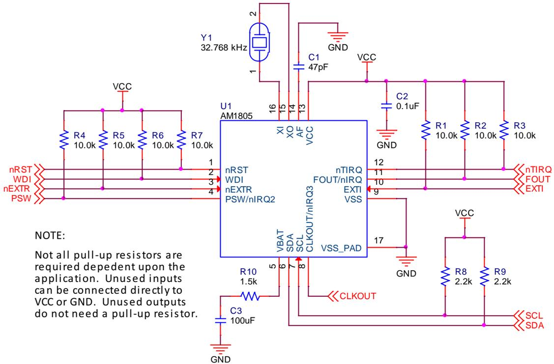
**Figure 8 – I<sup>2</sup>C Reference Schematic**
