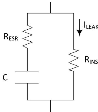
**Figure 6 – Low Frequency Capacitor Model**
