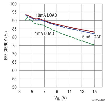
Figure 2. DC1754A Efficiency in Burst Mode Operation
