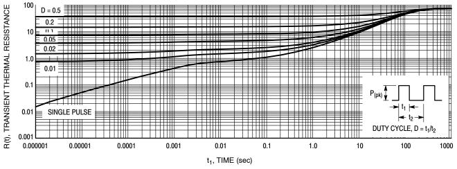
Figure 10. Thermal Response Junction-to-Ambient for MBRF2045CT
