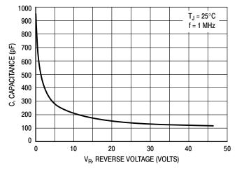
Figure 12. Typical Capacitance
