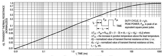
Figure 9. Thermal Response for MBR2045CT
