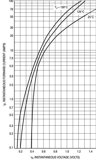
Figure 2. Maximum Forward Voltage
