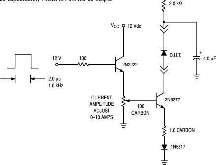
Figure 13. Test Circuit for dv/dt and Reverse Surge Current
