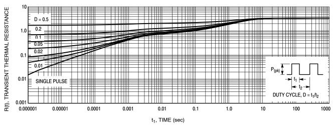
Figure 11. Thermal Response Junction-to-Case for MBRF2045CT
