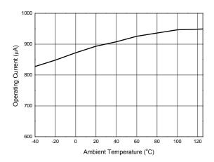
Start-up Current vs. Ambient Temperature
