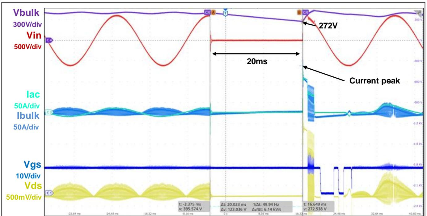
**Figure 34 Voltage drop of 10 ms at 2400 W**
