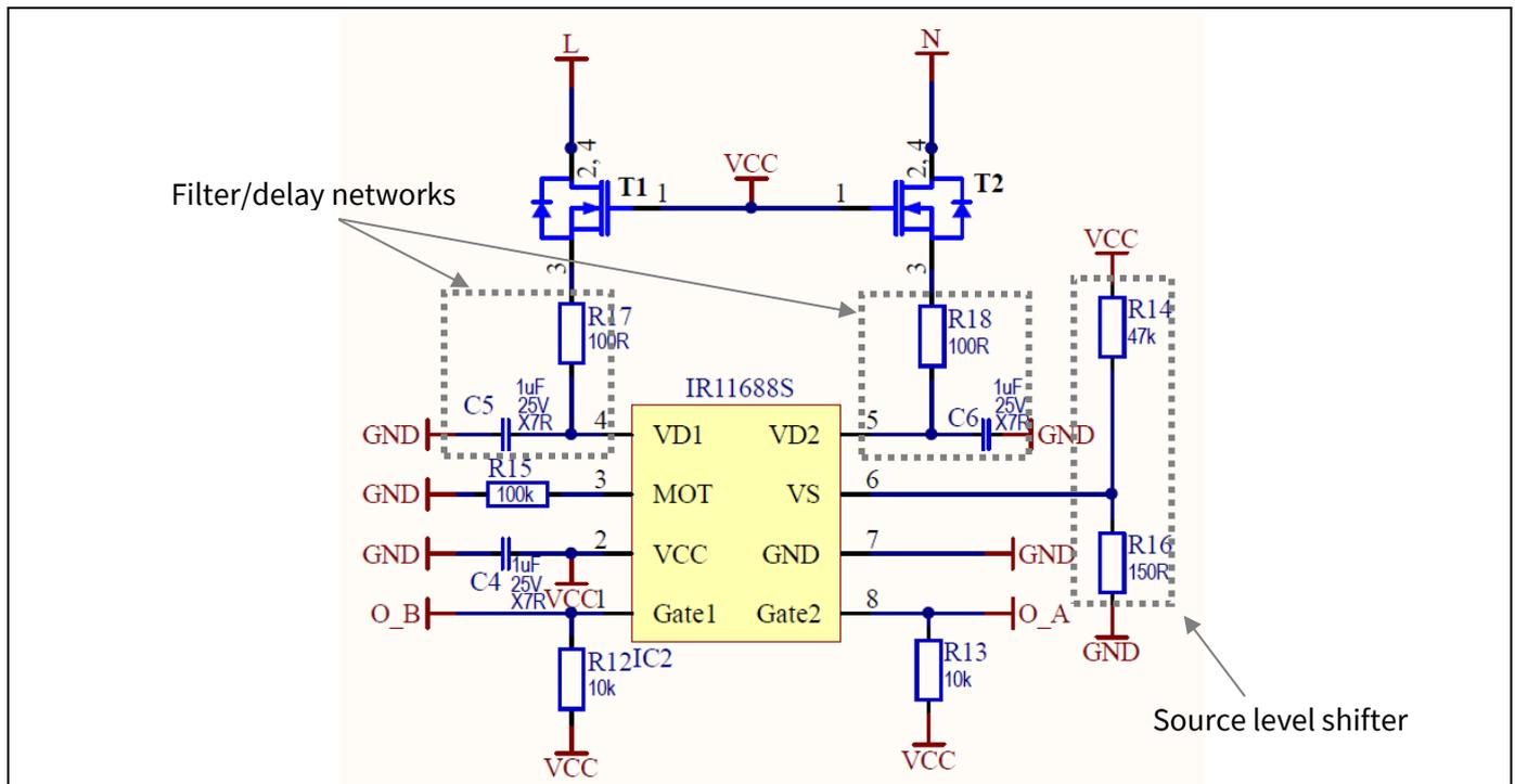
Figure 10 Adaptation of IR11688S for active-line rectification
