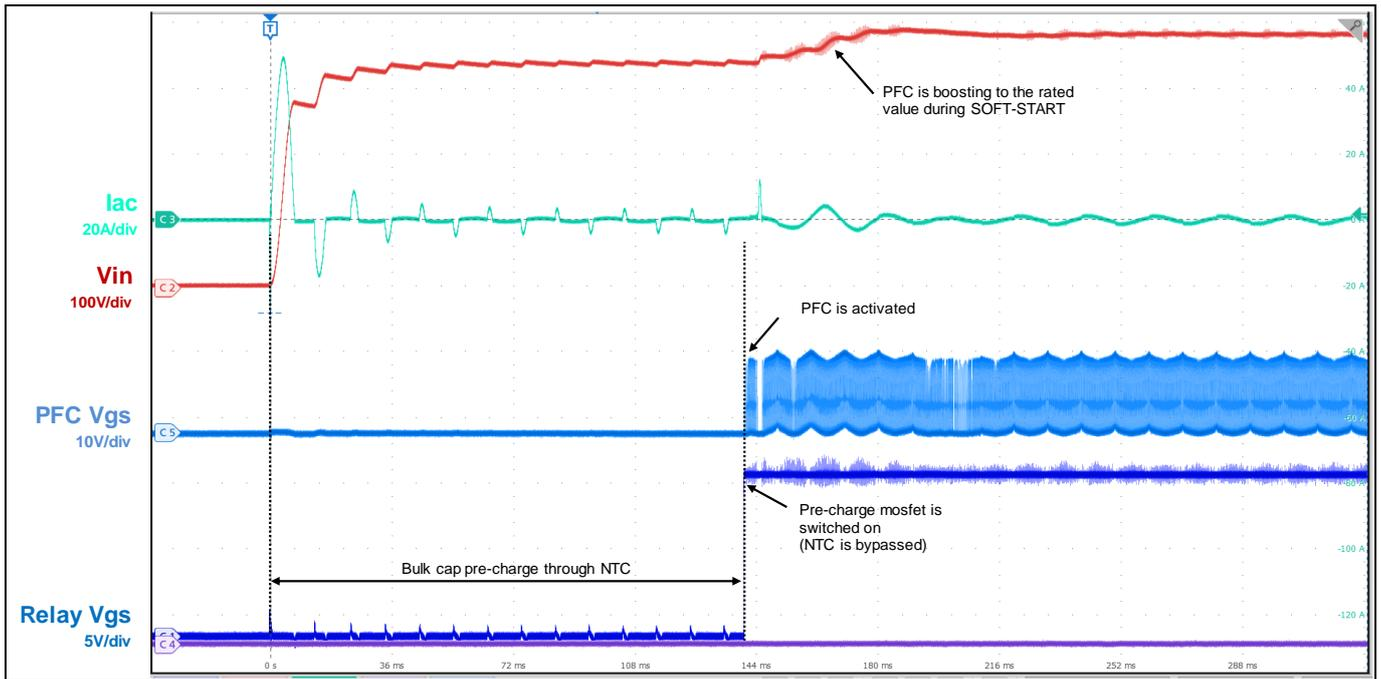
Figure 29 Pre-charge and PFC start-up at 250 V<sub>AC</sub>
