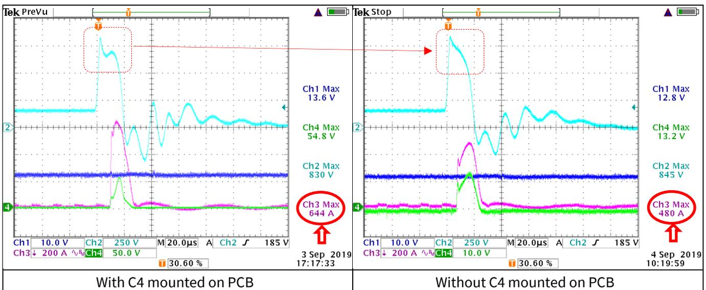
Figure 43 2 kV surge pulse BULK current
