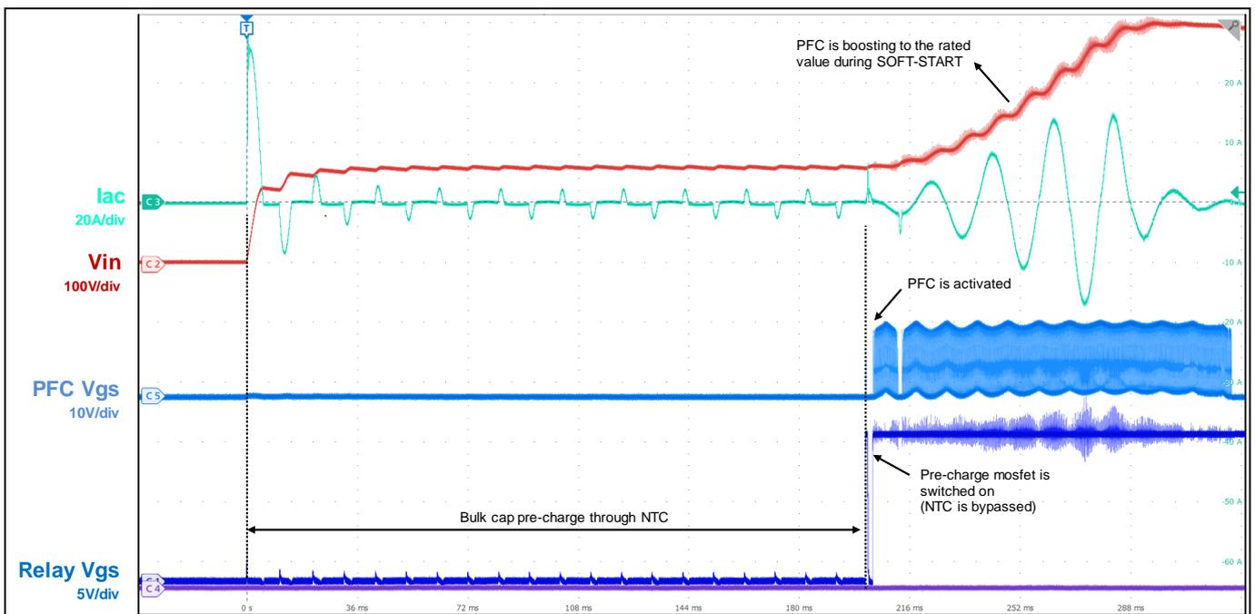
Figure 30 Pre-charge and PFC start-up at 120 V<sub>AC</sub>
