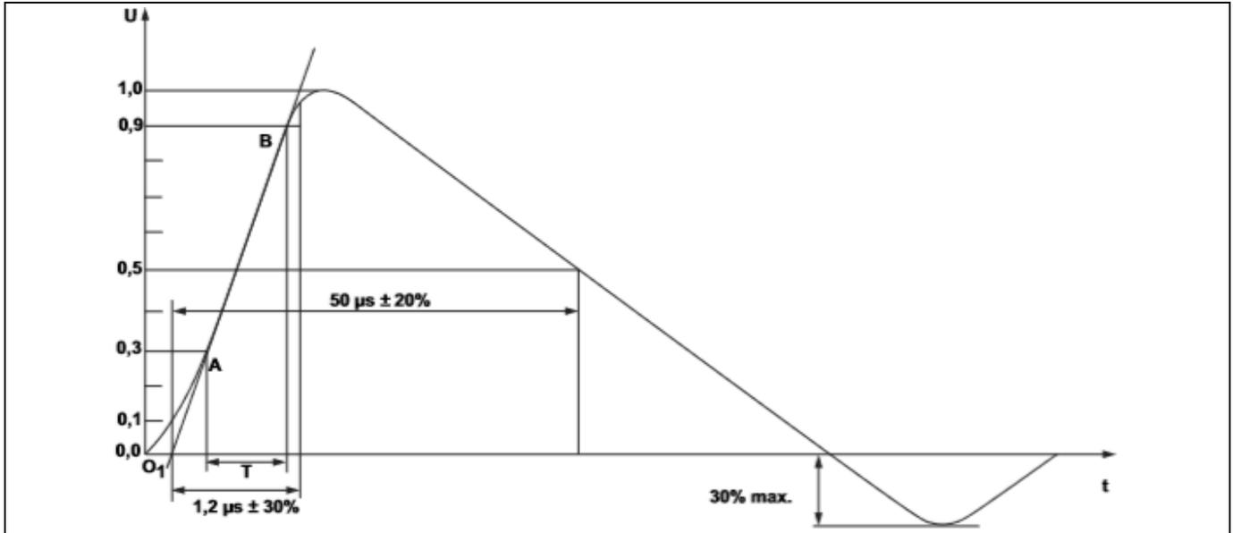
Figure 36 Surge voltage waveform according to IEC 61000-4-5
