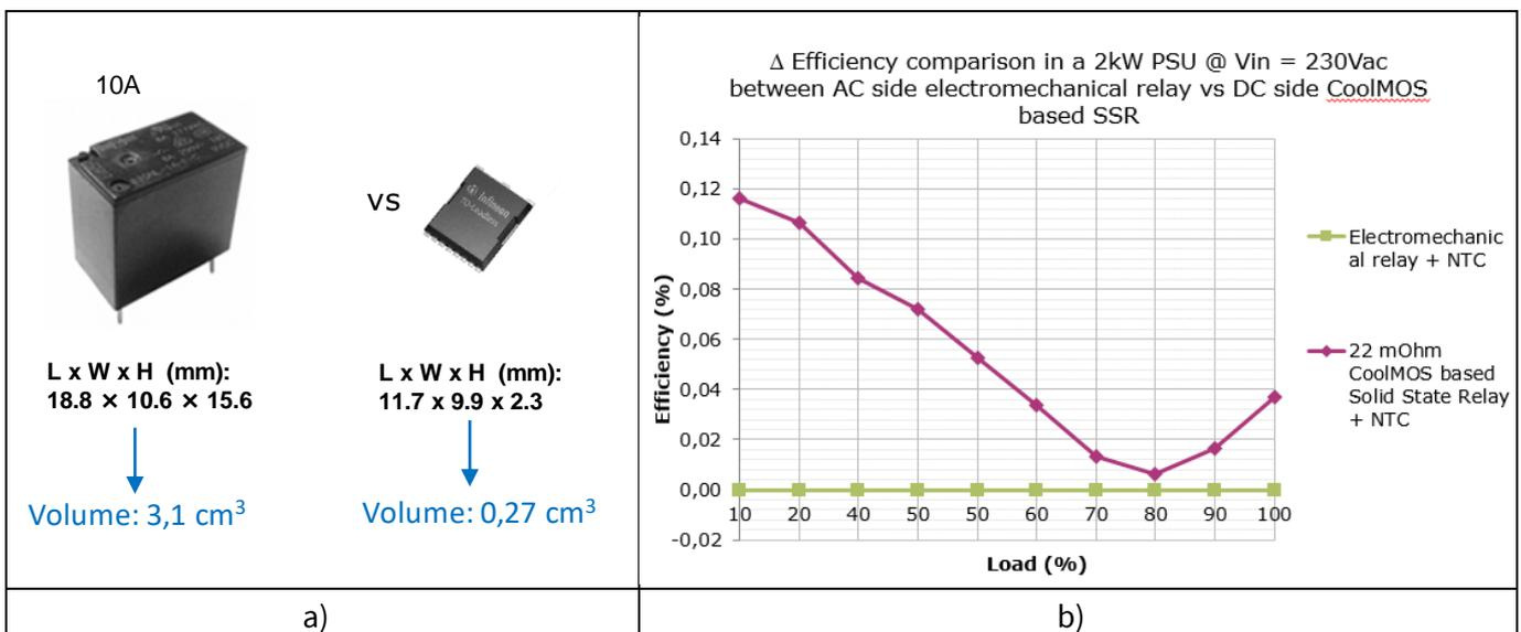
Figure 27 Size (a) and efficiency (b) comparison between standard mechanical relay at AC-side and CoolMOS™-based solution at DC-side
