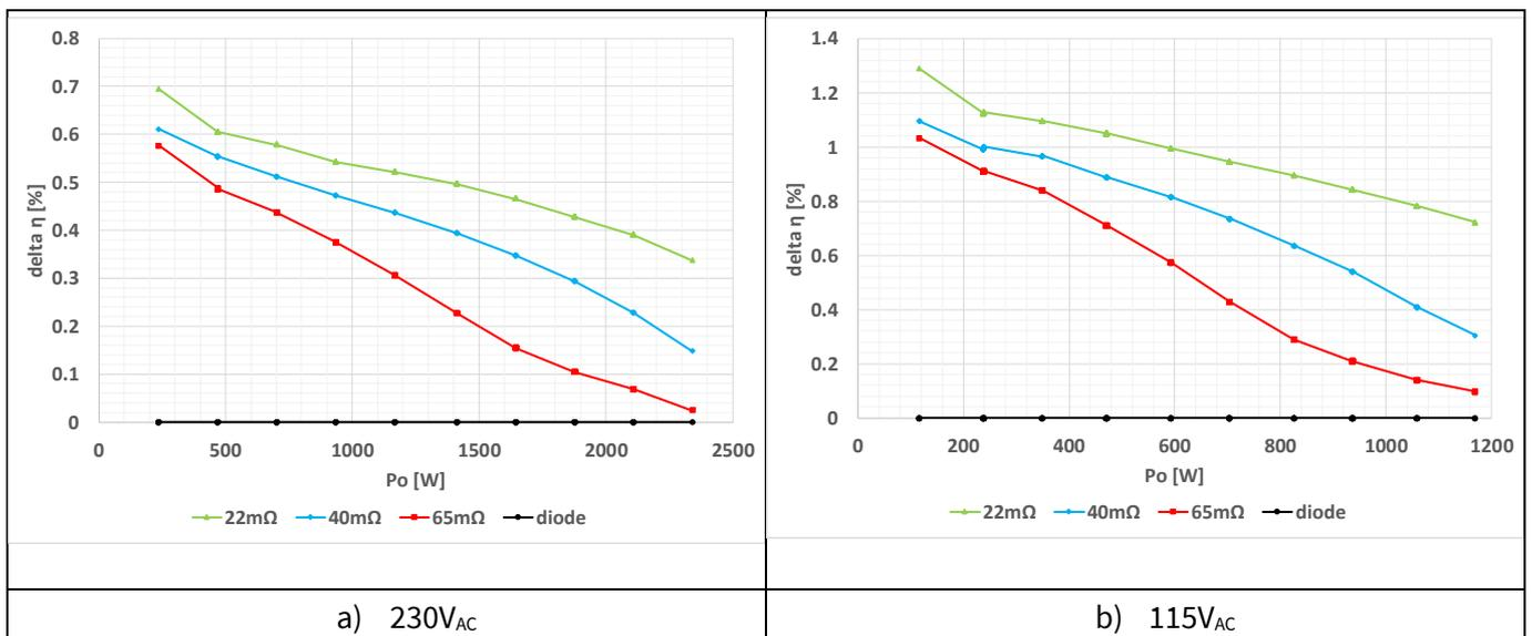
Figure 20 Delta efficiency test result of EVAL\_2K4W\_ACT\_BRD\_S7: comparison between passive and active bridge at different R<sub>DS,ON</sub>
