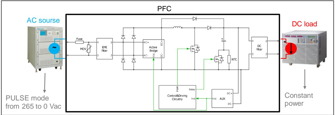
Figure 31 Test-bench for voltage drop-out emulation
