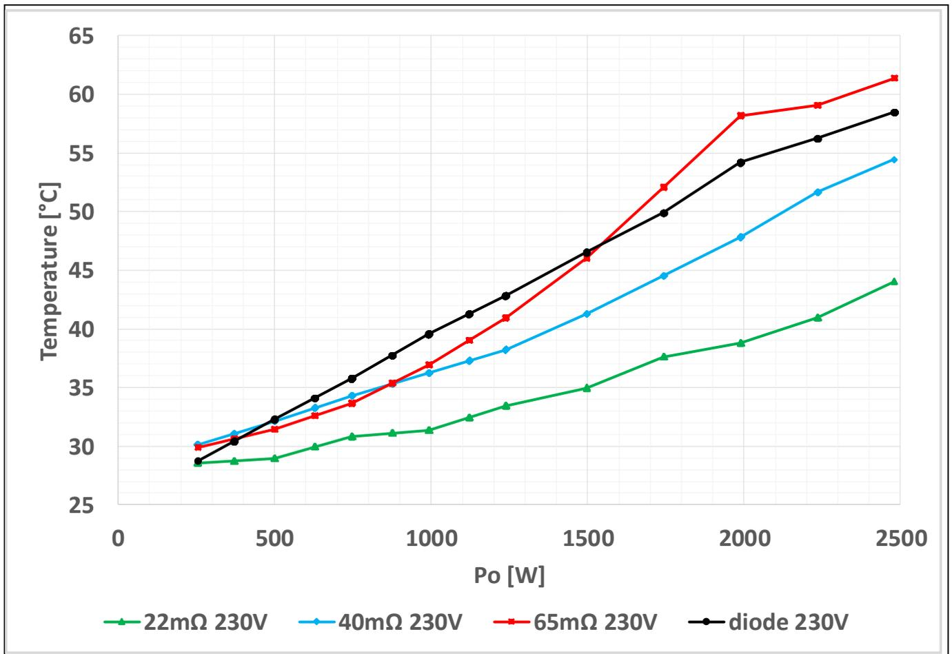
Figure 22 Bridge temperature measurements of EVAL\_2K4W\_ACT\_BRD\_S7 at nominal high-line
