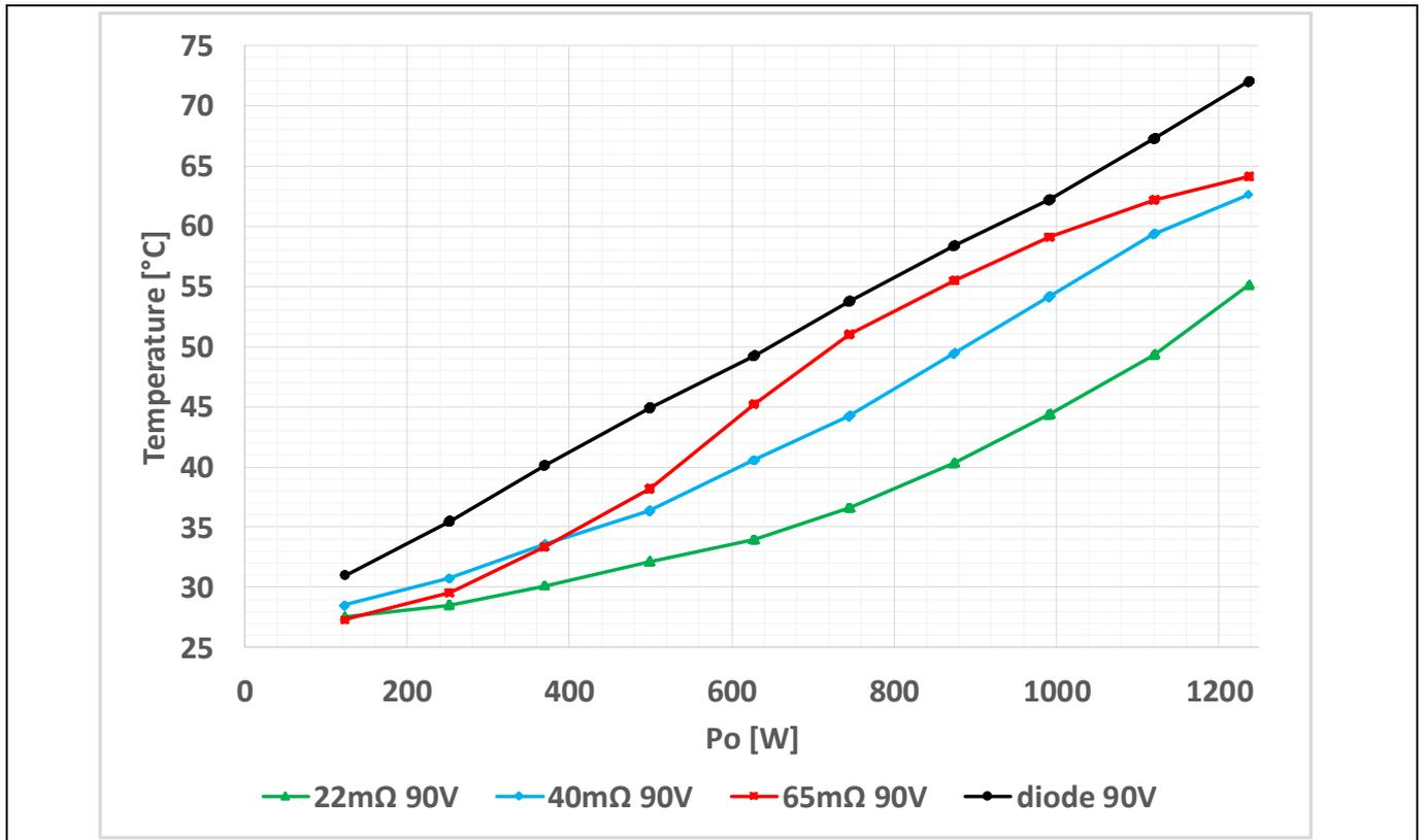
Figure 23 Bridge temperature measurements of EVAL\_2K4W\_ACT\_BRD\_S7 at minimum low-line
