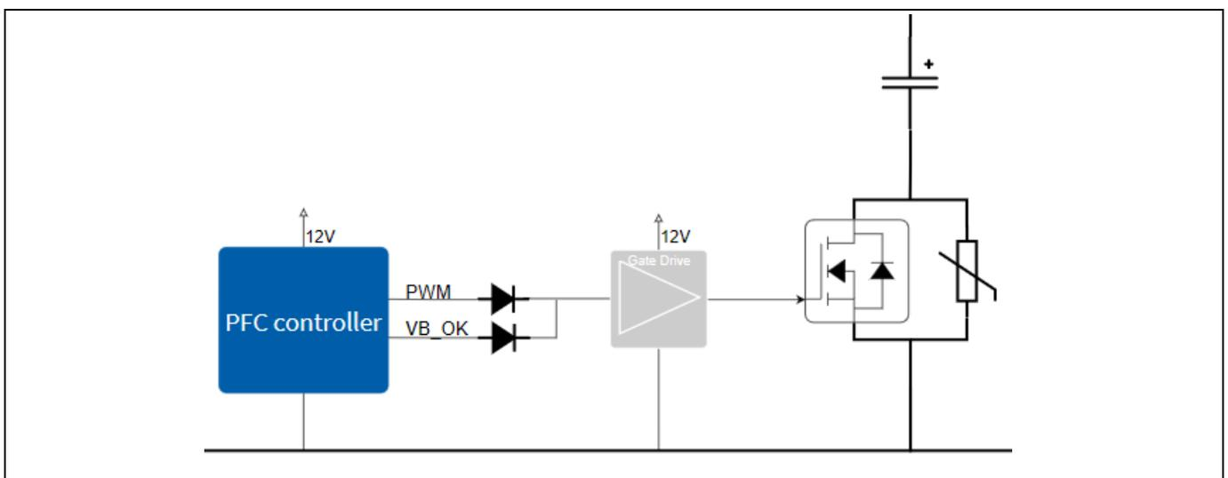
**Figure 28 Control network of the pre-charge MOSFET**
