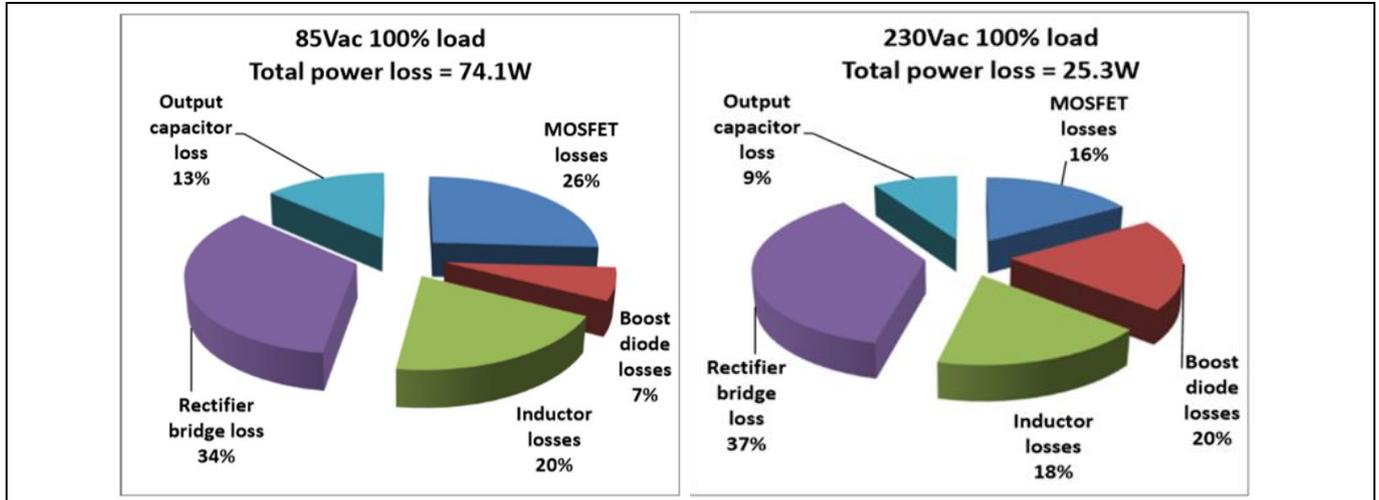
Figure 13 Power dissipation of power devices with a 1000 W PFC circuit at 85 V<sub>AC</sub> and 230 V<sub>AC</sub>
