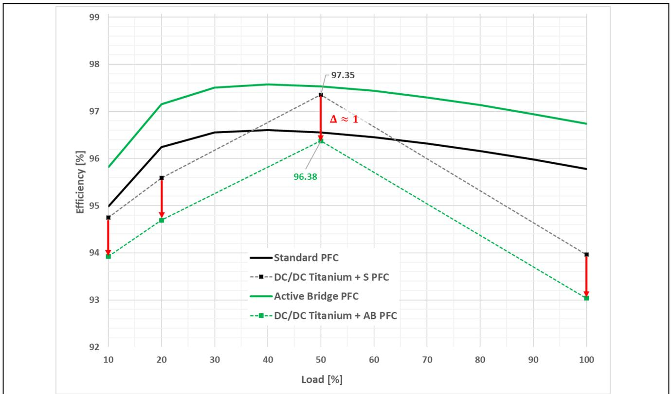
Figure 3 Reduction of DC-DC efficiency requirements for an 80 PLUS Titanium design thanks to the active bridge (at 115 V<sub>Ac</sub>)
