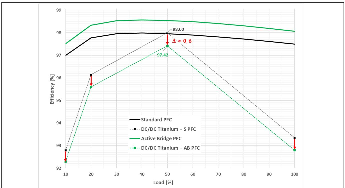
**Figure 2 Reduction of DC-DC efficiency requirements for a PLUS Titanium design thanks to the active bridge (at 230 V<sub>Ac</sub>)**
