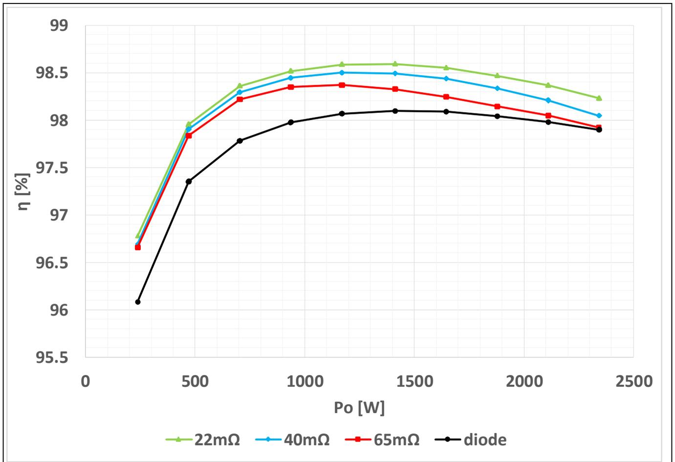
**Figure 18 Efficiency test result of EVAL\_2K4W\_ACT\_BRD\_S7 with 22 mΩ (green line), 40 mΩ (light blue), 65 mΩ (red) active-bridge line rectification and with only the diode bridge (black) at 230 V<sub>AC</sub>**
