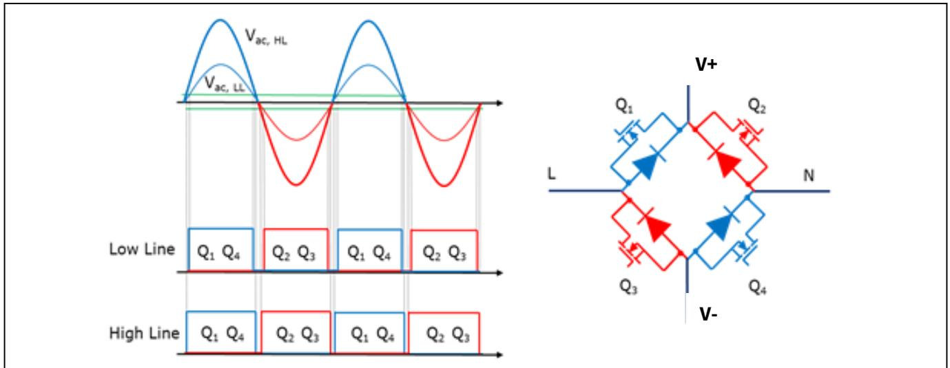
Figure 7 Control concept of the active-bridge line rectification
