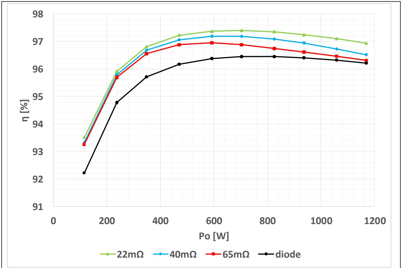
Figure 19 Efficiency test result of EVAL\_2K4W\_ACT\_BRD\_S7 with 22 mΩ, 40 mΩ, 65 mΩ full-wave active-bridge line rectification and without active bridge (passive) at 115 V<sub>AC</sub>
