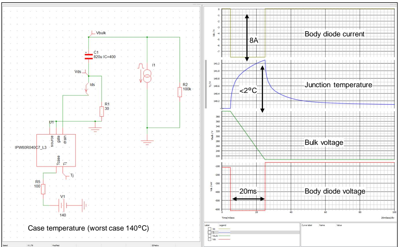
Figure 35 Simulation in case of relay CoolMOS™ body diode conducting during voltage drop-out
