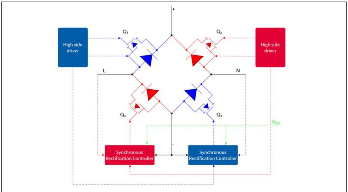
Figure 9 Second approach based on the SR controller
