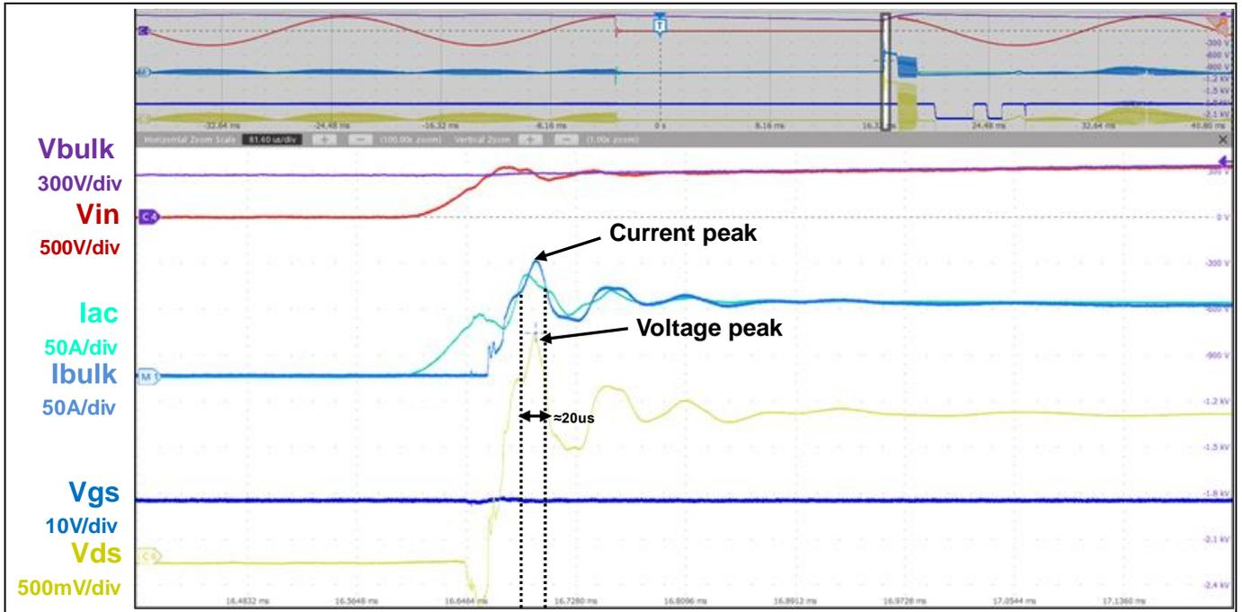
**Figure 33 Zoom: voltage drop of 20 ms at 1800 W**
