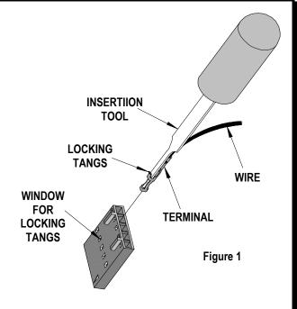
**Note**: Please do not forcefully insert, insert on an angle, or insert with twisting action. It may damage the tool or the housing.
