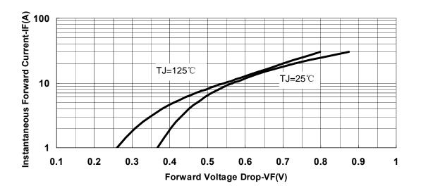
Fig.3-Typical Instantaneous Forward Voltage Characteristics
