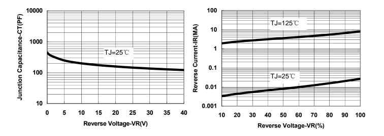
Fig.1-Typical Junction Capacitance
