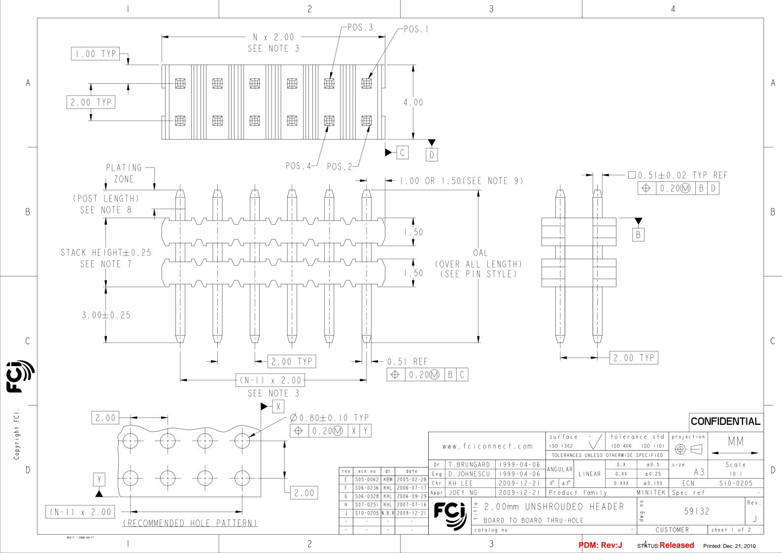
$S = 0.38 \mu m GOLD$ ON CONTACT AREA 0.38 µm GOLD ON TAIL
