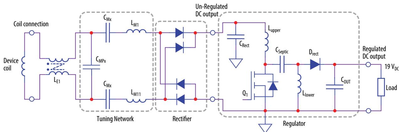
Figure 2: Schematic diagram of the EPC9514 demo board.
