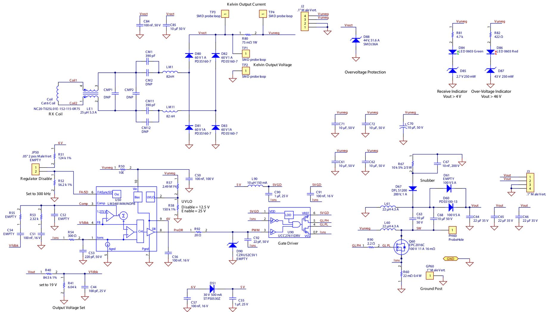
Figure 4: EPC9514 Receiver schematic.
